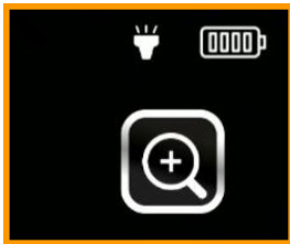
Fig. 8-4 A white icon is displayed when the white light flashlight is in use
