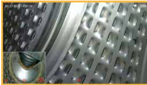
Fig. 8-29 Live Image With the Side View Camera as the Primary Image and the Front View Camera as the Secondary Image
